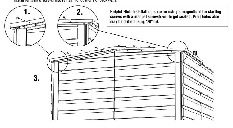
From inside the shed, install four **Screws (AA)** into the roof, two on each side wall.
